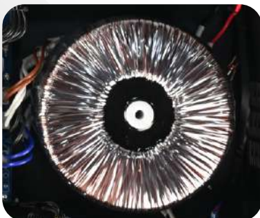
Large Toroidal Copper Transformer for Stable Power Supply and low noise
